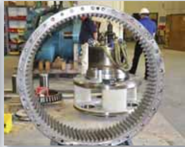
Wind turbine outer gear in the enXco operations and maintenance facility in Riverside County
