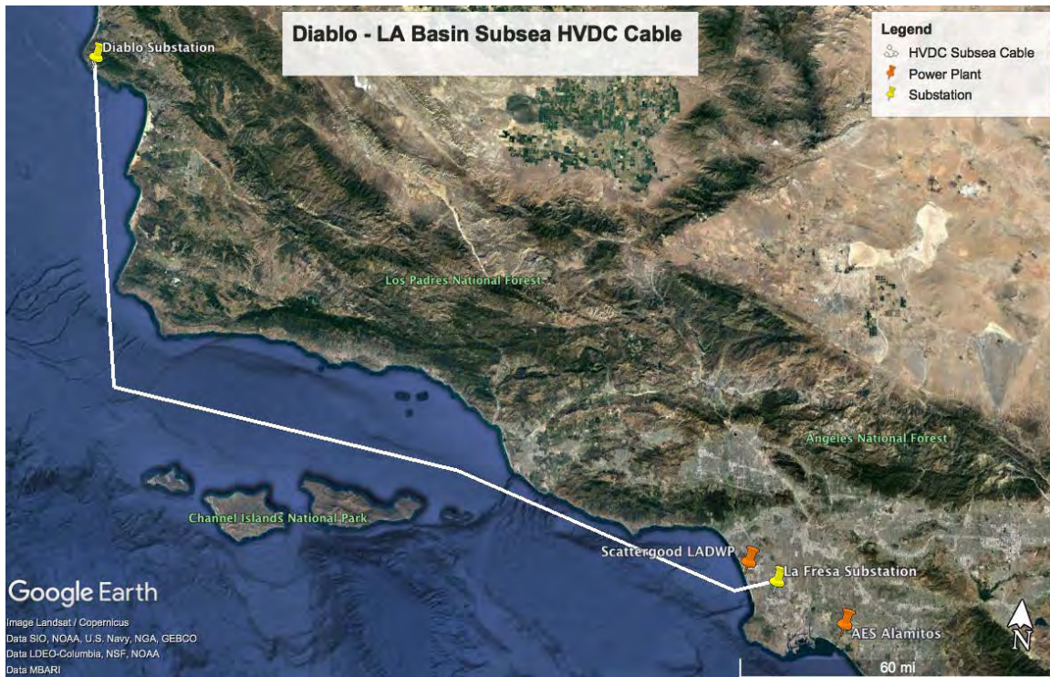
Figure 6. Diablo Canyon to LA Basin Subsea HVDC cable conceptual map
