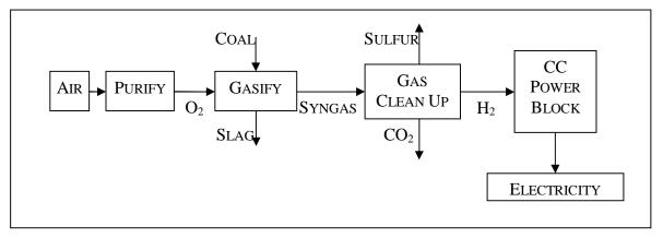
A schematic diagram of the IGCC process is shown in Figure 5-8.
