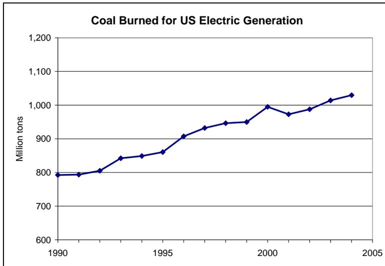
**Figure 5-5** U.S. coal consumption for electric generation.<sup>7</sup>
