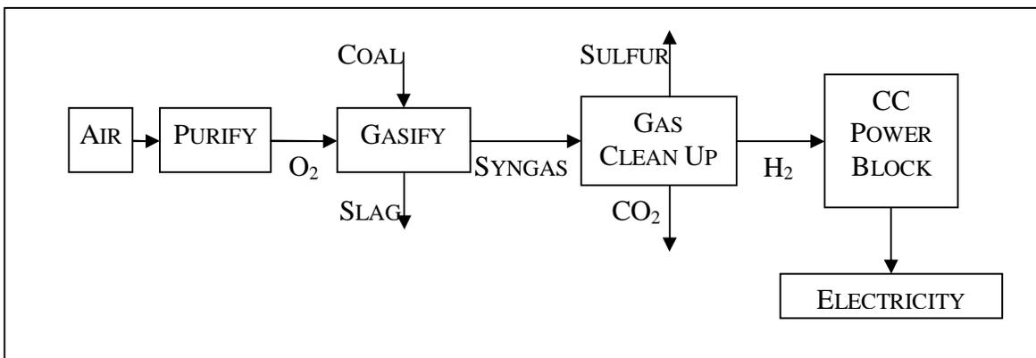
**Figure 5-8** Schematic diagram of coal IGCC process
