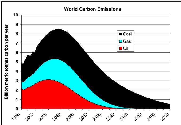
**Figure 6-3** Carbon emissions from fossil fuel burning projected by Hubbert-type analysis
