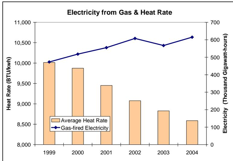
**Figure 4-10** Gas required to generate one kilowatt-hour of electricity (“heat rate”) and electricity generated by gas-fired power plants
