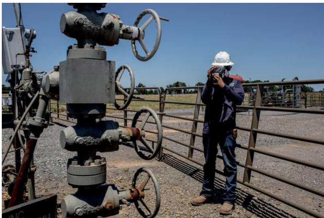
A technician searching for methane leaks with an infrared camera in Damascus, Ark. Andrea Morales for The New York Times
