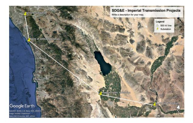
The North Gila — Imperial Valley #2 500 kV Line Project is part of the Southern Area Reinforcement. The following figure provides a schematic diagram of the transmission system in the area. As shown in the figure, the project scope includes a new 500 kV circuit between North Gila and Imperial Valley substations, estimated at 97 miles. The CAISO estimates that the proposed project will cost approximately \$340 million, with an in-service date of June, 2028.
